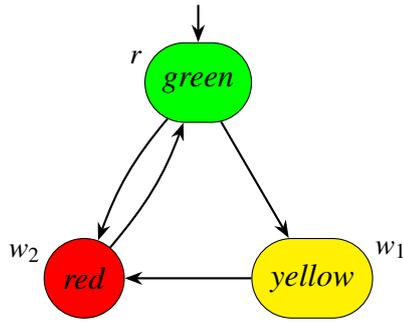
Figure 1.1: Kripke model  $\mathcal{M}$  of a three signal traffic light.
